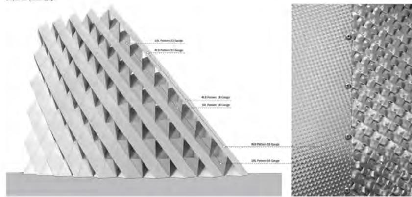
Figure 8: Final boards showing the integration of the tetrahedron and octahedron geometry to the global geometry of the facade.
