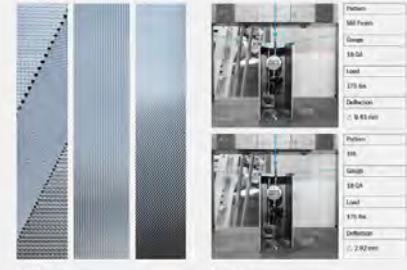
This process identifies the very character of rigidized stainless steel that makes it a "high performance material": one that does not change its properties but has "selected and designed" properties exhibiting extremely high strength in stiffness and particular reflectivity. The process also identifies the first scale, within the proposed part-to-whole relationship governing the design of the research proposal.
