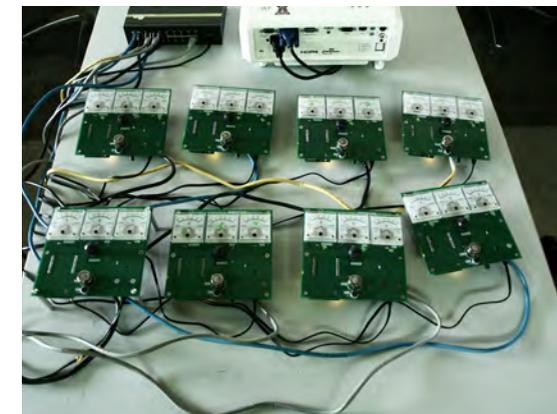
Right: Sensor boards connected to network for testing prior to installation
