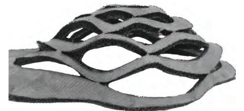
Figure 2: (Left) 2D pattern laser cut in Concrete Canvas. (Right) Popped-up Concrete Canvas shell prototype.
