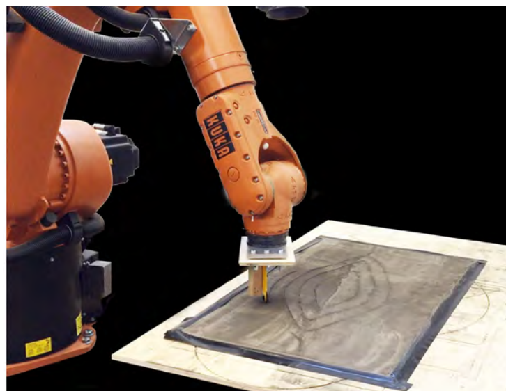
Figure 7: (Left) Robot cutting pattern in concrete. (Right) 1.0 x 0.7 x 0.7 m popped-up prototype.
