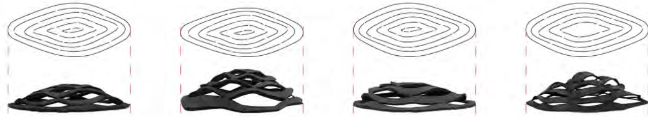
Figure 6: Comparison of geometric differences in the 3D pop-up surfaces; product of changes in boundary conditions and cutting patterns.
