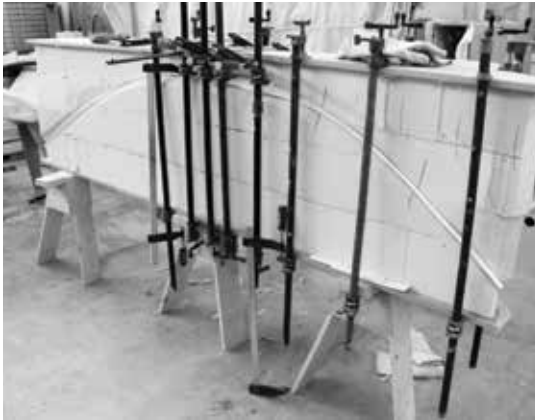
Figure 7: Male and female mold required at areas of intense curvature, such as the creases.
