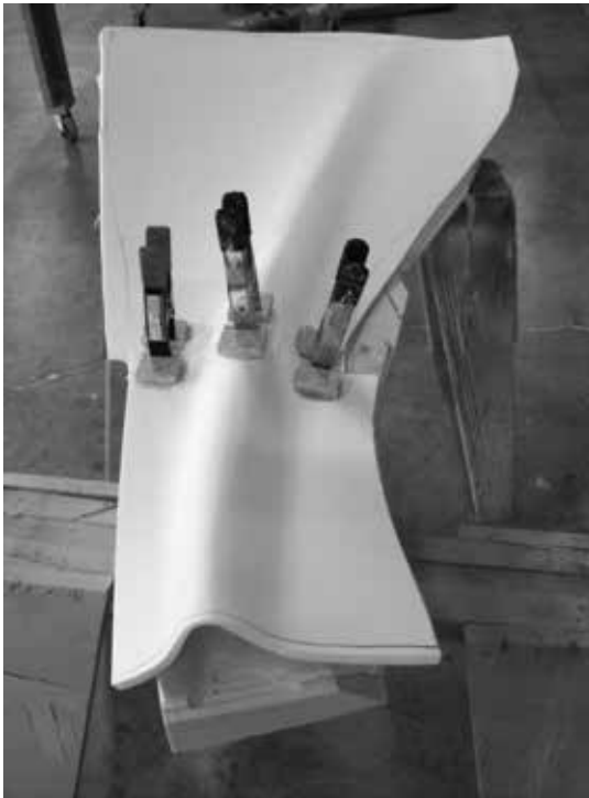
Figure 8: Seaming of smaller sections to form a larger panel.
