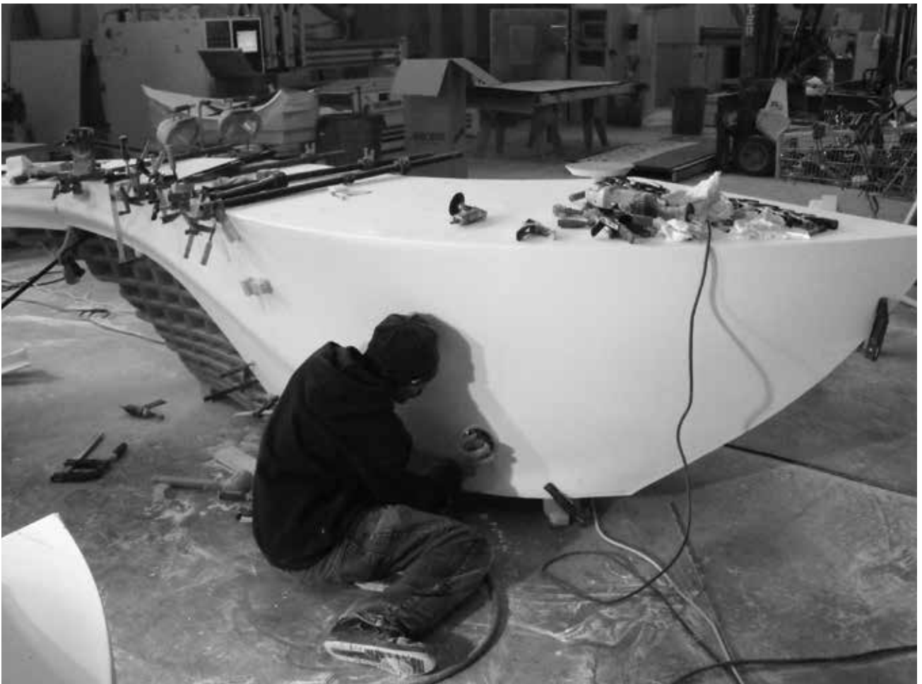
Figure 9: Hand polishing of HI-MACS to buff out all seams into a single surface.
