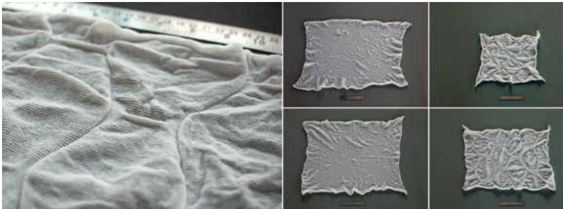
Figure 9: Custom knitted textile with differentiated structures, significantly varying material size and performance (Sean Ahlquist, 2012)
