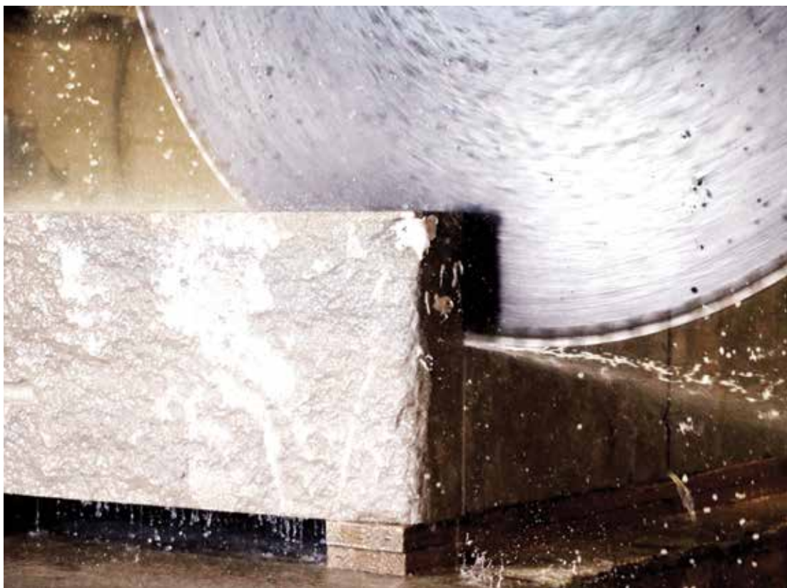
Figure 4: Cutting Indiana limestone from slabs to blanks.
