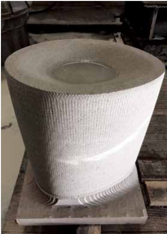
Figure 13: Initial drum study for the Shape Deformation method, which led to improvements in the drum face geometry and milling strategy.
