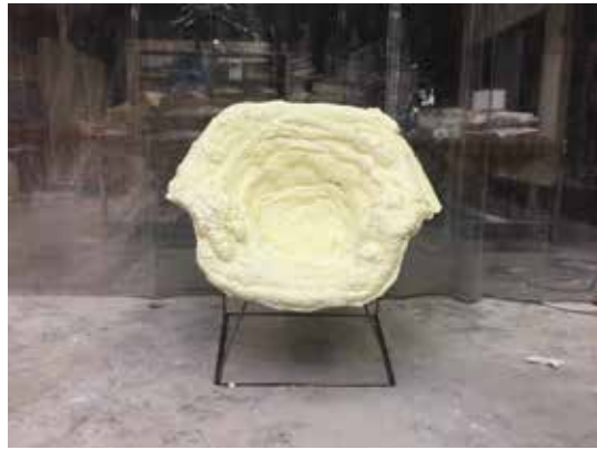
Figure 3: (clockwise from top left) Textile formwork for Eames molded fiberglass chair; foam-sprayed backing side of the Womb Chair; both molds prepared and sealed for GFRC casting.
