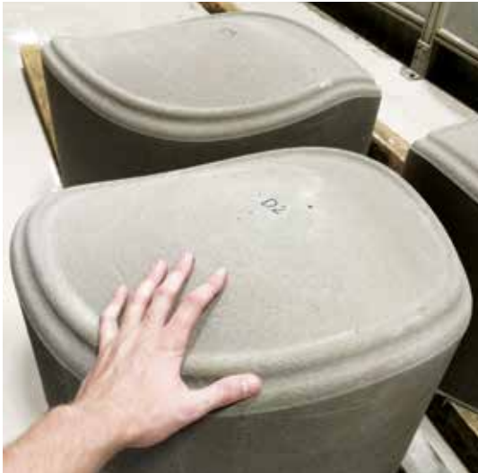
Figure 9: Filleted drum seam as seen from the column exterior.
