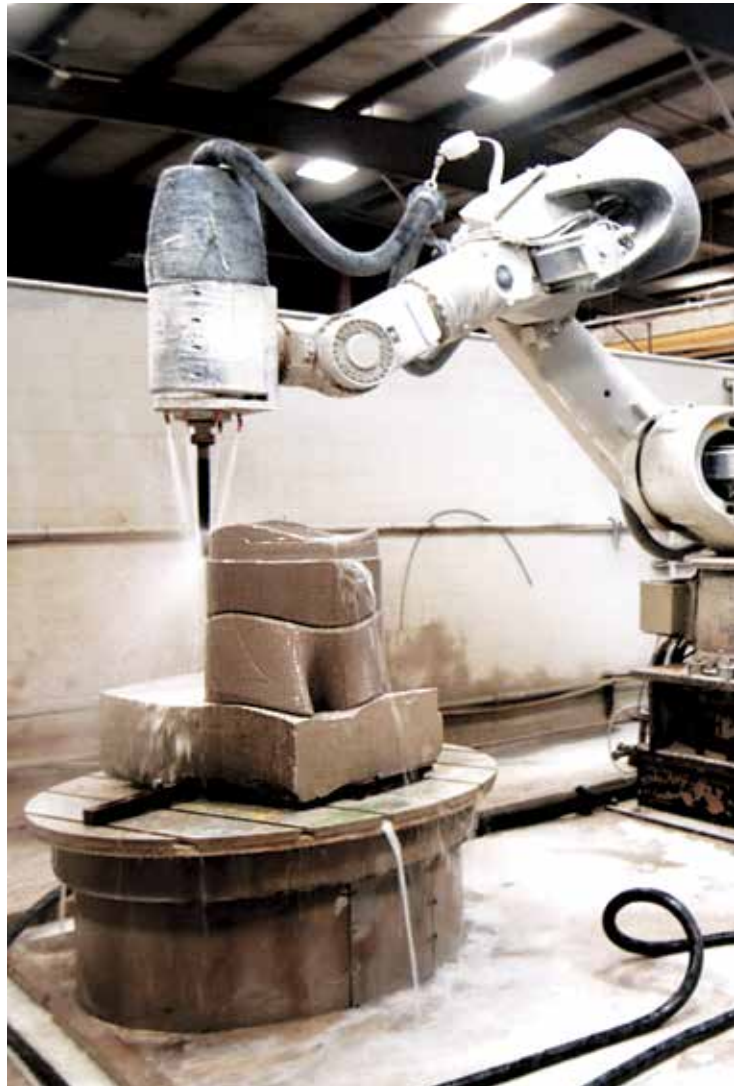
Figure 6: Key Index Strategy – roughing operation of stacked drum.
