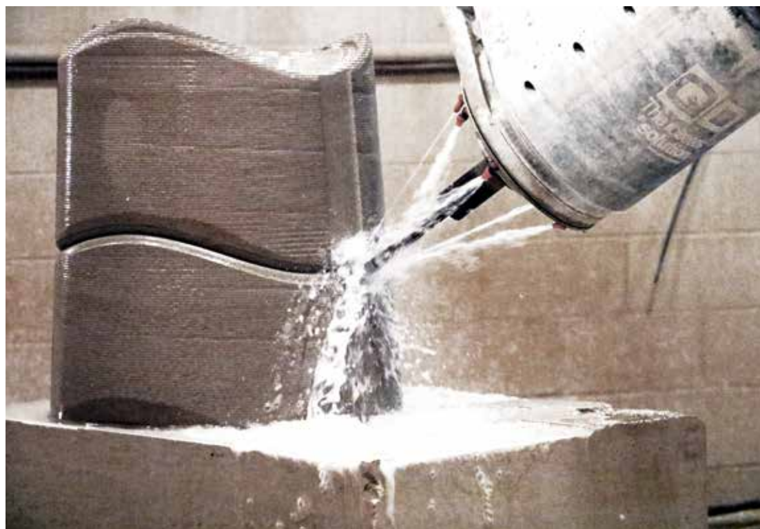
Figure 5: Finish milling of exterior surface utilizing a seven-axis toolpath.
