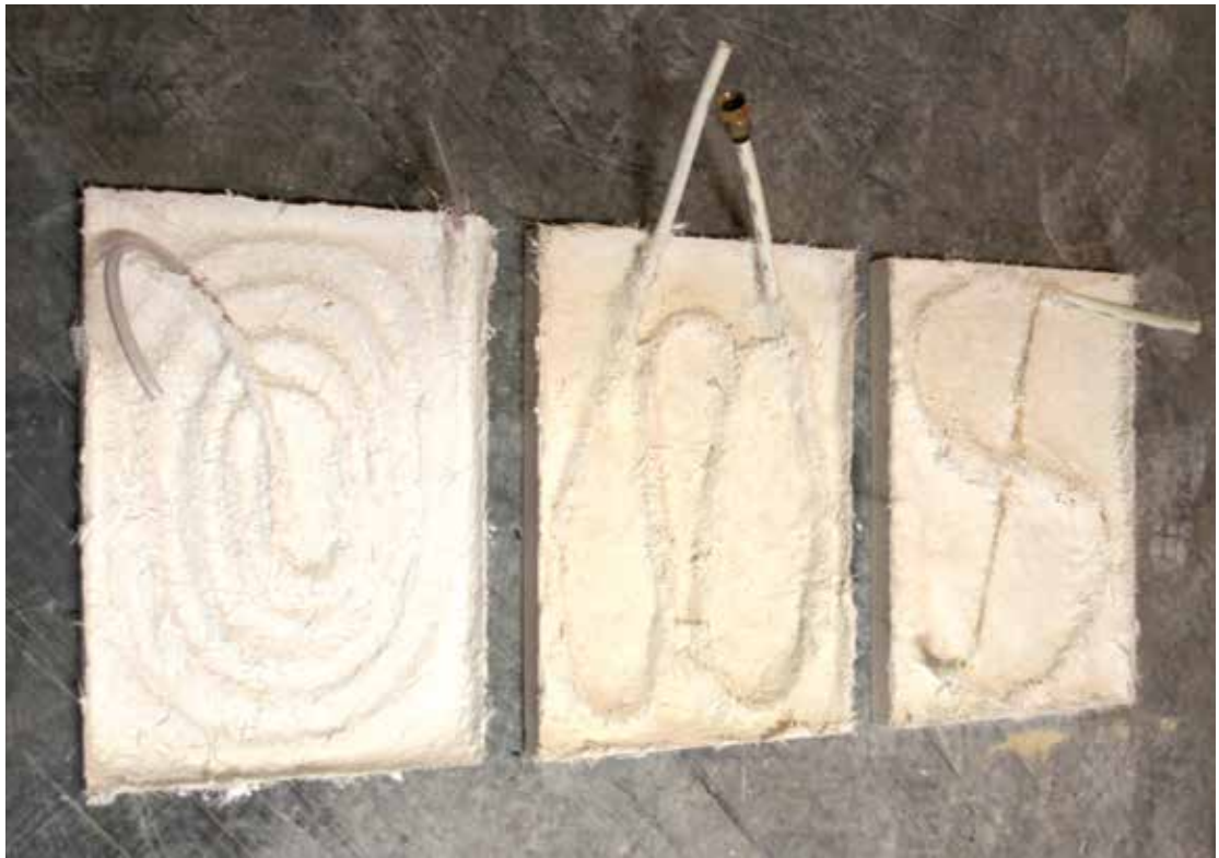
Figure 5: Material prototypes with variable density of hydronic tubes.
