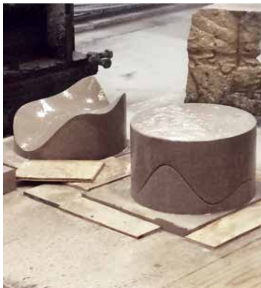
Figure 14: Flip milling key strategy prototype. The dramatic amplitude of the drum faces confirmed rotational stability as compared to a flat drum face.
