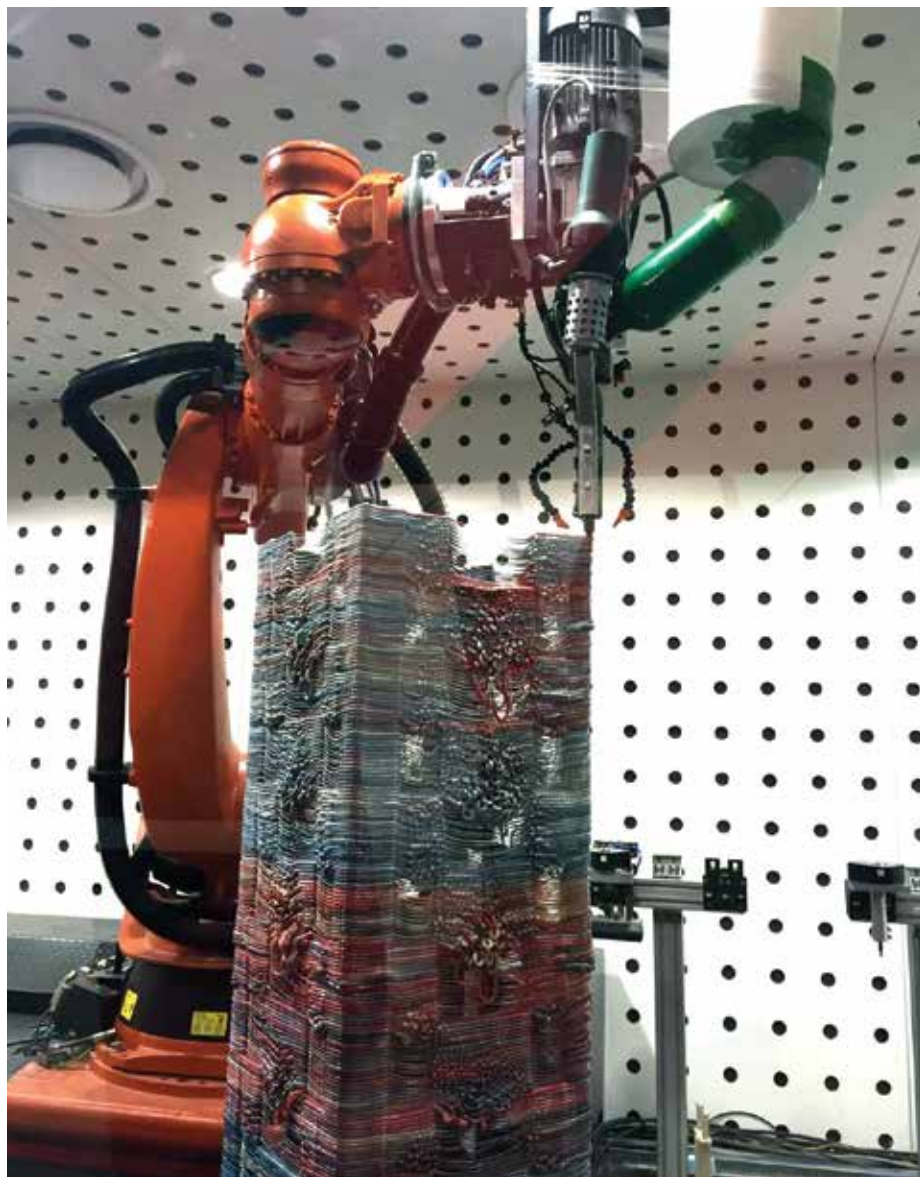
Figure 7: The robotic setup, consisting of a six-axis industrial robot and an extrusion head.
