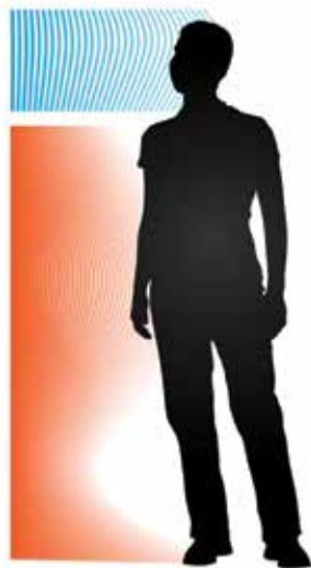
Predominantly warm environment diagram cooling > face cooling > chest cooling > abdomen cooling > thigh (most effective to provide comfort) ↓ (least effective)
