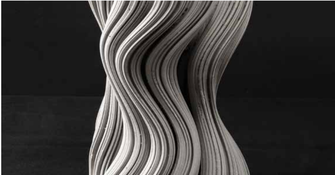
Figure 14: Prototype for an architectural concrete element cast in Submillimetre Formwork. - DBT, ETH Zürich, 2017.
