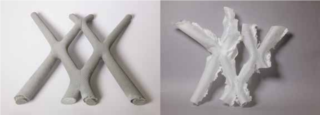
Figure 11: Concrete component displaying high-resolution texture (left) after the Submillimetre plastic formwork has been removed (right). - DBT, ETH Zürich, 2017
